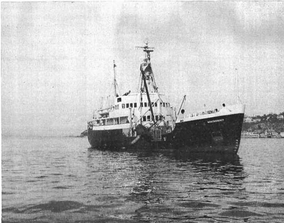
CCGS Montmorency, lighthouse supply and buoy vessel, is shown laying buoys in the St. Lawrence, an annual task. (Department of Transport Photo)
