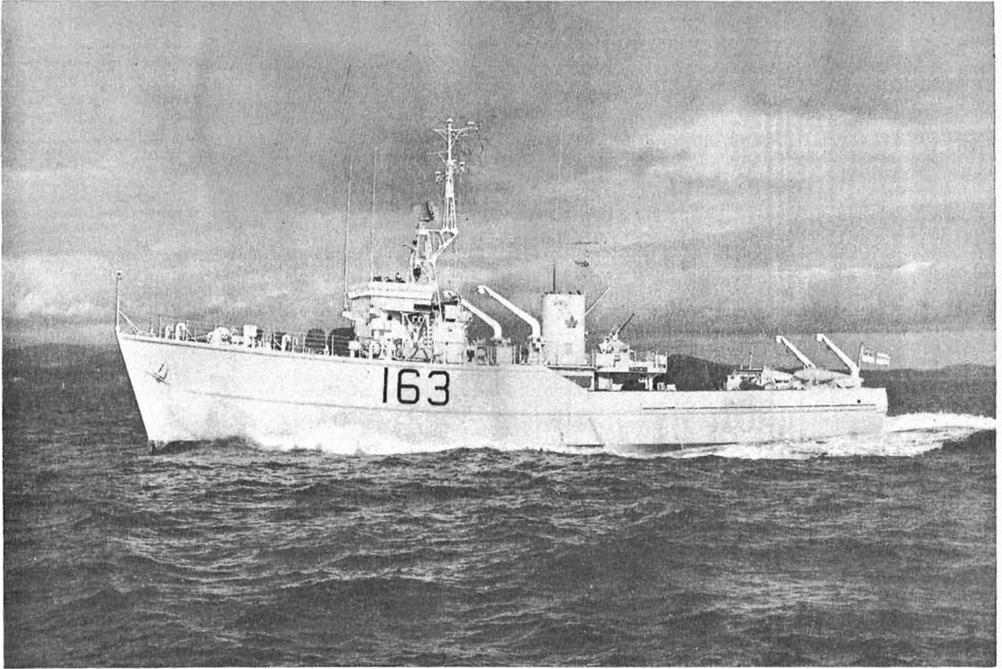
HMCS Miramichi, is one of the RCN's postwar Bay class minesweepers. These wooden sweepers are equipped to deal with a variety of mines. (E-43508)
