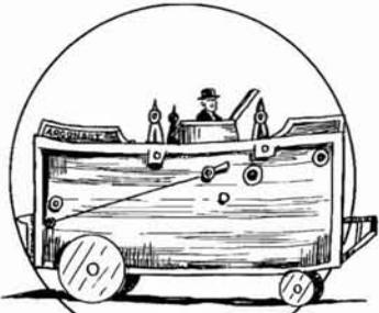
'ARGONAUT JUNIOR'... FIRST SIMON LAKE SUBMARINE. 14 FEET IN LENGTH AND FILLED WITH COMPRESSED AIR, SHE MOVED ALONG THE SEA BED ON MANUALLY CRANKED WHEELS.
