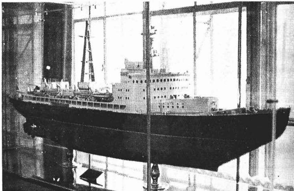
Here are two views of a model of the Russian nuclear-powered icebreaker, *Lenin*, launched late in 1957. Her engines will develop from 44,000 to 56,000 horsepower and she will have three propellers, giving her a maximum speed of 18 knots. It is reported that the *Lenin* will be able to steam for a full year without refuelling and that her daily fuel consumption will be five ounces.
