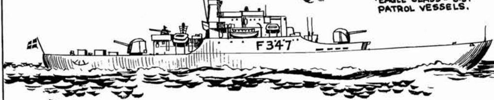
DANISH CORVETTE 'TRITON' CLASS. (ITALIAN BUILT) - 760 TONS, 2 3 IN. GUNS. BUILT FOR PATROL AND ESCORT DUTIES.
