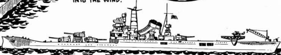
JAPANESE CRUISER 'TSUSHIMA' CLASS (9000 TONS)...CARRIED 11 TO 13 AIRCRAFT IN HANGAR IN STERN WITH 2 CATAPULTS.
