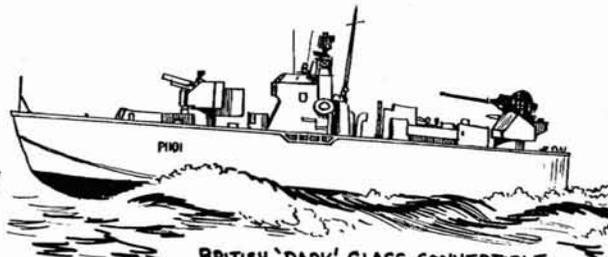
BRITISH 'DARK' CLASS CONVERTIBLE MOTOR TORPEDO/MOTOR GUN BOATS (DELTAIC ENGINES). AS GUNBOATS THEY CARRY 1 4.5 IN. GUN, AND 1 40 MM A.A. GUN. AS M.T.B.s THEY CARRY 4 21 IN. TORPEDO TUBES AND ONE 40 MM A.A. GUN. SPEED IS APPROXIMATELY 40 KNOTS.
