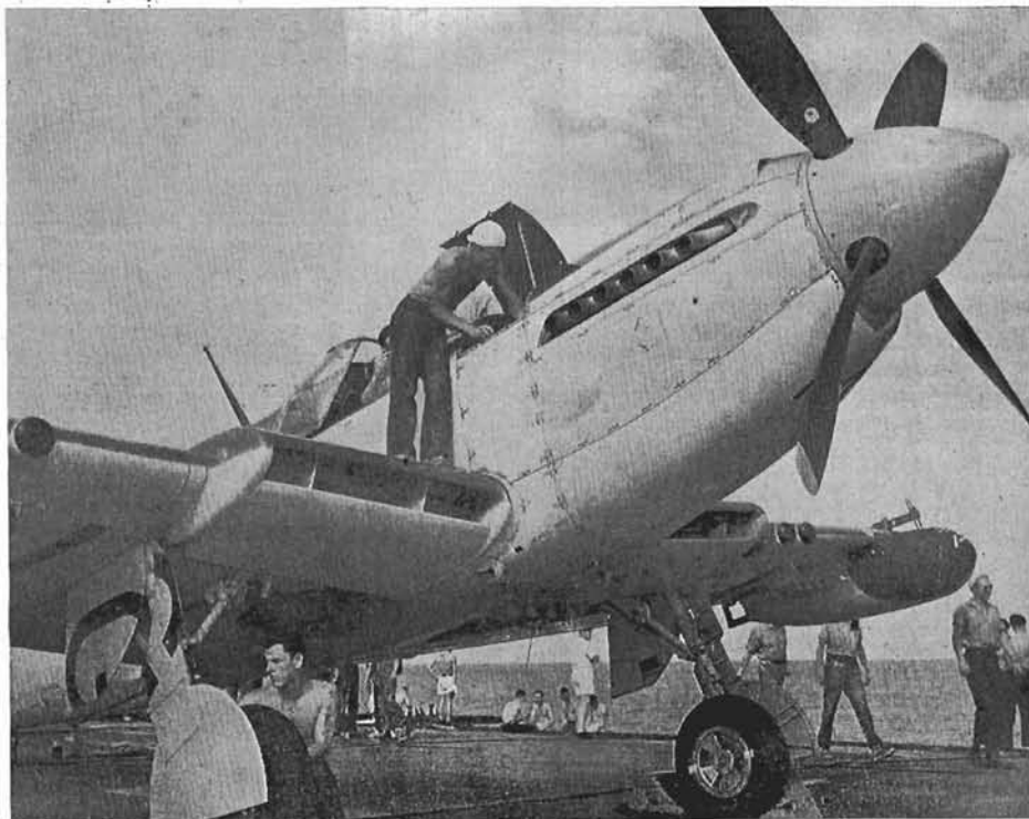
It was the air maintenance men who "kept 'em flying" during the spring cruise. Here a Firefly's maintenance crew carries out the daily inspection during a lull in flying activity. AB Douglas Gascho examines the undercarriage and AB Edmond Poirier checks the oil consumption. (Mag-1336).
